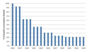
From 2018 onwards, the EU F-Gas Regulation [EU 517/2014] creates massive cuts in the consumption of HFCs in the EU. This reduction scheme, known as the HFC phase-down, is based on a quota system. Quotas are expressed in CO<sub>2</sub> equivalent (kg x GWP).
